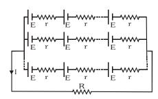
Total internal resistance of the circuit  $r_{net} = \frac{nr}{m}$
