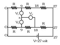
$$\frac{x-9}{R_v} + \frac{x-9}{R_v} + \frac{x-18}{R_v} = 0 \Rightarrow x = 12 \therefore V_3 = 6 \text{ volt}$$
