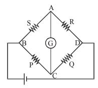
If P is slightly increased, potential of C will decrease. Hence current will from A to C. If Q is slightly increased, potential of C will increases, hence current will flow from C to A.
